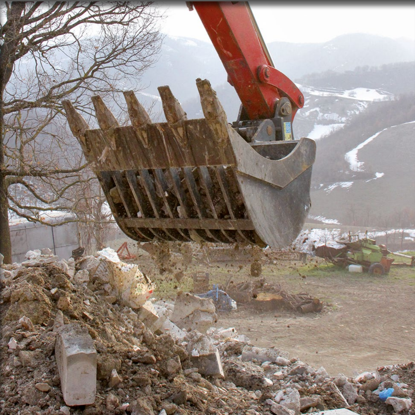
THE SKELETON BUCKET IS DESIGNED TO SORT STONES AND AGGREGATE MATERIALS. THE SIEVED MATERIAL'S SIZE DEPENDS ON THE DISTANCE AMONG THE GRIDS.
