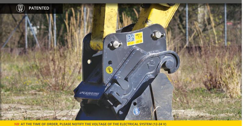
THE PATENTED SEMI-AUTOMATIC CW AUT'O'LOCK QUICK COUPLER ENABLES THE FAST LOCKING AND UNLOCKING OF THE ATTACHMENTS, CONSIDERABLY REDUCING THE TIME FOR THEIR REPLACEMENT. IT IS PROVIDED WITH A SEMI-AUTOMATIC SYSTEM THAT REQUIRES THE MANUAL INTERVENTION WHEN THE TOOL
