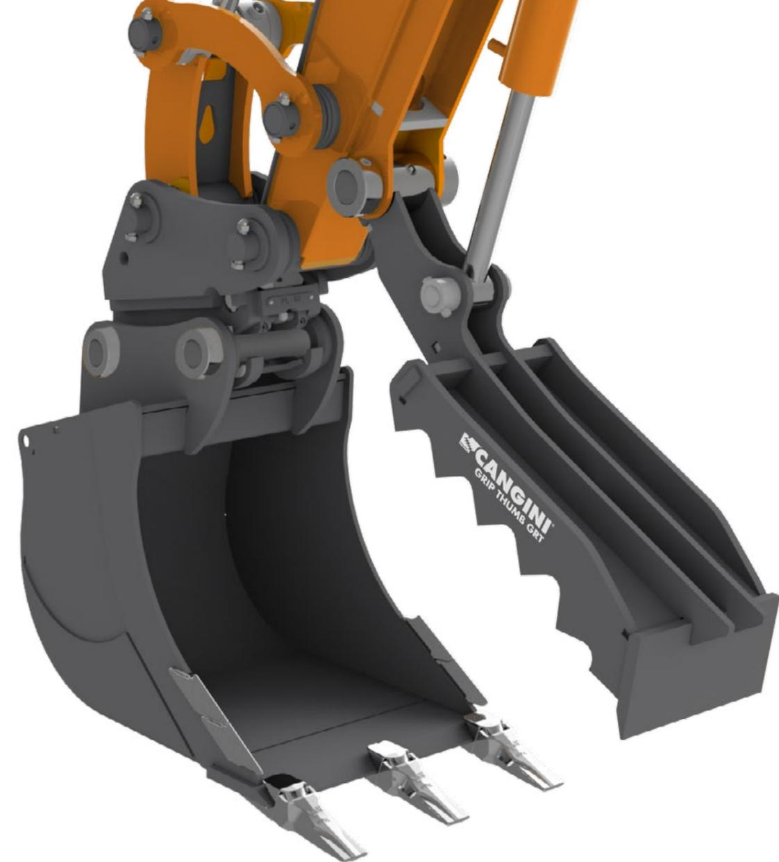
SOUDE SUR LE BRAS, LE POUCE GRT CANGINI FACILITE LA PRISE DE MATÉRIAUX ROCHEUX, TRONCS ET AUTRES, FAISANT OFFICE DE PINCE. UNE FOIS COMPLÈTEMENT RÉTRACTÉ, IL PERMET LE FONCTIONNEMENT NORMAL DU GODET, FACILITANT AINSI LE TRAVAIL DE L'OPÉRATEUR.
