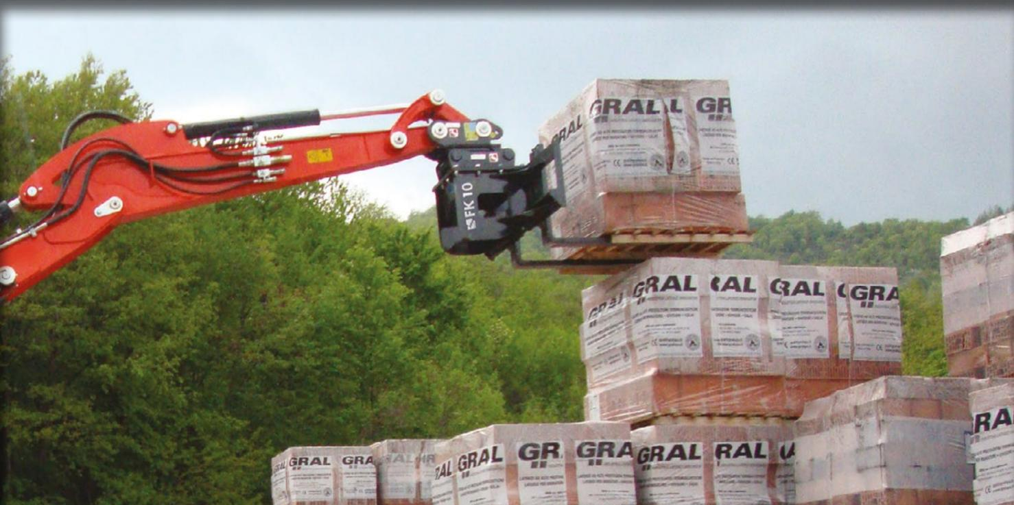
CETTE CONFIGURATION PERMET L'ACCROCHAGE AUX PELLES ET REND LE TABLIER APPROPRIÉ POUR LA MANUTENTION DES CHARGES DANS DE ZONES DURES D'ARRIVER AUTREMENT. CEPENDANT, IL FAUT VÉRIFIER QUE LA PELLE EST HOMOLOGUÉE POUR LE LEVAGE COMME L'EXIGE LA DIRECTIVE MACHINES.
